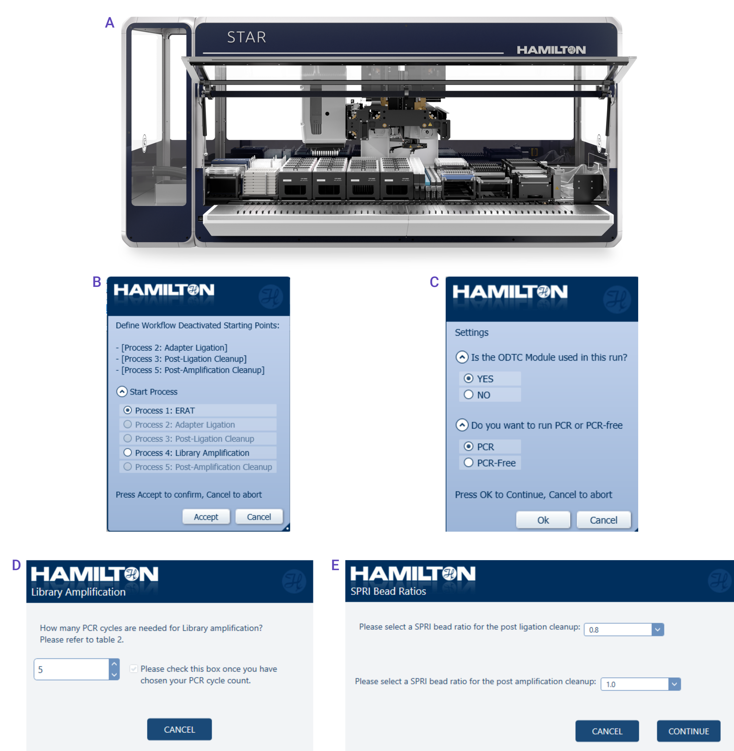
Figure 1. Dynamic User Options. (A) The Hamilton Microlab NGS STAR MOA enables flexibility and speed utilizing both its MPH and 8-independent channels. The Watchmaker DNA Library Prep script includes (B) dynamic runtime user options for safe start/stop points, (C) run conditions, (D) PCR cycles, (E) SPRI bead cleanup ratios, and more.
